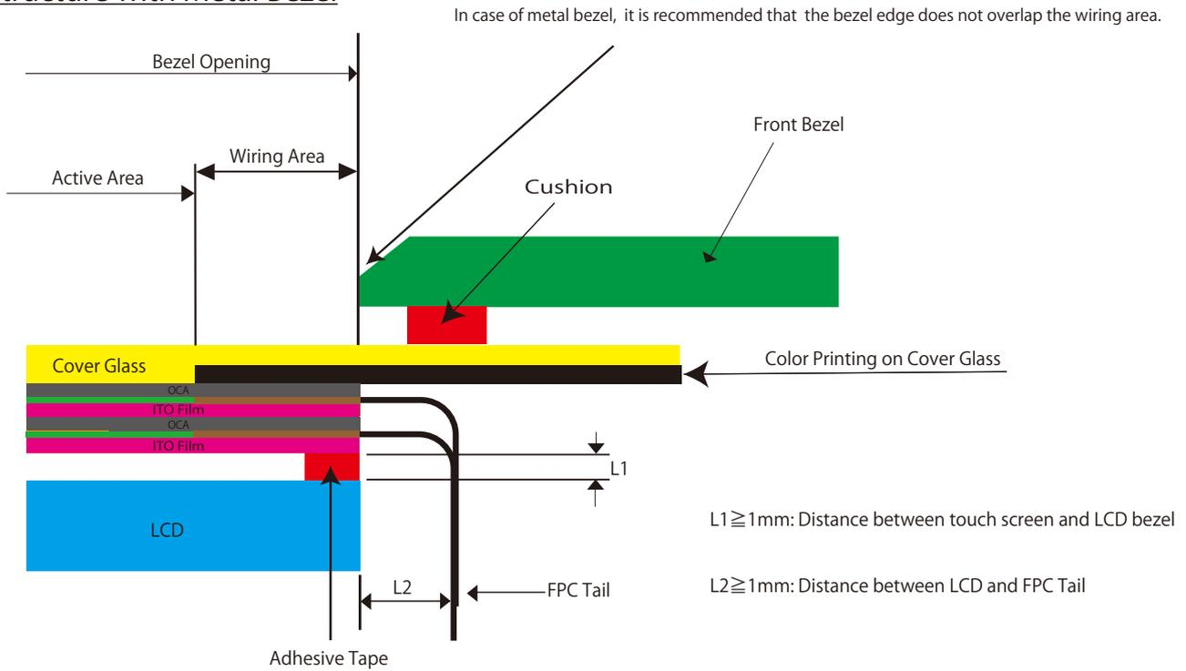
Structure with Resin Bezel
